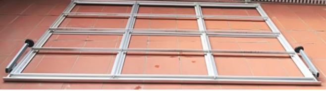
Figure 3: Aluminium chassis embedding the 12 rectangular double-chamber PVC panels (see Fig. 2).
