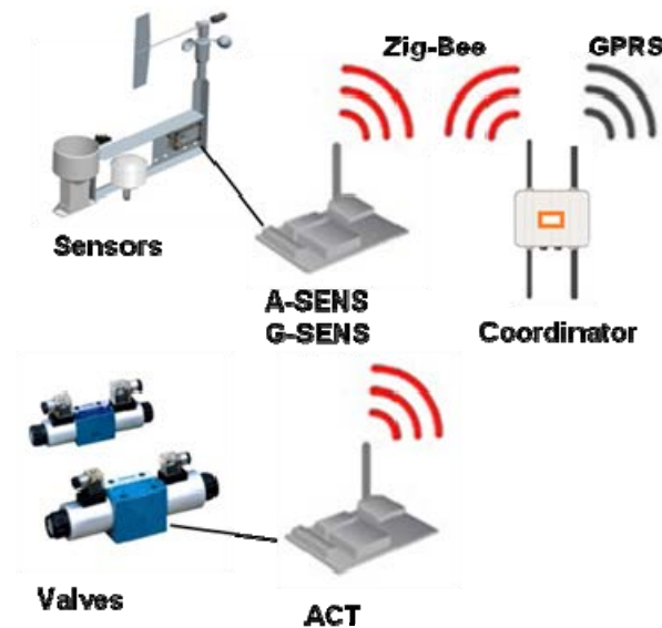
Fig. 3. Field unit: logic structure.
